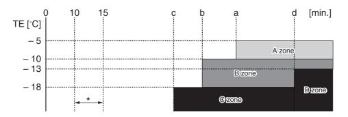
\* From 10 minutes to 15 minutes after a heating operation started, the minimum value of TE is stored in memory as TEO and the minimum temperature of TO as ToO.
